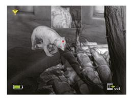
Picture-in-Picture improves accuracy by providing a 2x magnified image of the reticle area at the top of the display. It helps to zoom in on a target while retaining the rest of the field of view visible.
