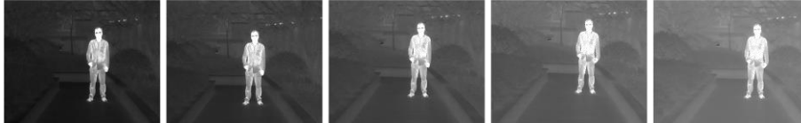
Figure 3-4 Adjust Brightness in White Hot Mode
